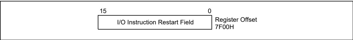
Figure 33-5. I/O Instruction Restart Field
