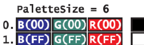
Fig. 33.44: Palette Structure of a Black & White, One-BitImage
